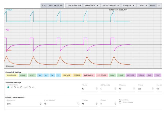
Fig. 1 VentSim© software main features> The figure shows the simulation environment of VCV ventilation in the main modality offered by the software.
