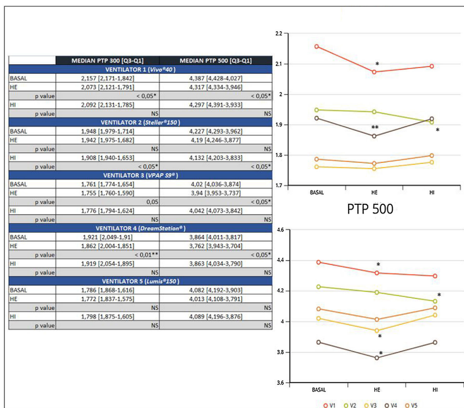
Figure 2 Comparative representation of median PTP300 and PTP500 according to NIV device and type of humidification. HE: external humidifier; HI: internal humidifier; V1: Vivo®40; V2: Stellar®; V3: VPAP S9®; V4: DreamST®; V5: Lumis® 150; *: p < 0.05 ; ** p < 0.01 . NS: non-significant.
