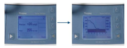
**Figure 2** DTDS show us objective numeric parameters like de suction pressure and air leak flow. It represents these parameters in graphics that can be downloaded.
